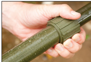
Rotate stem nuts and rinse again to ensure grit has been removed.
