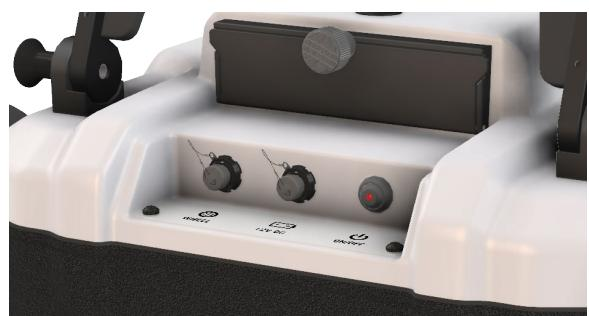
The batteries are found under the black lid. You can hot-swap the batteries, one battery at time, during a measurement. This will keep you going without the need to shut off the equipment when changing the batteries during a survey.
