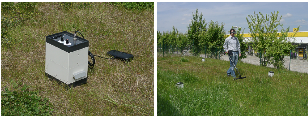
Figure 60: Placement of the VLF emitter on a site
