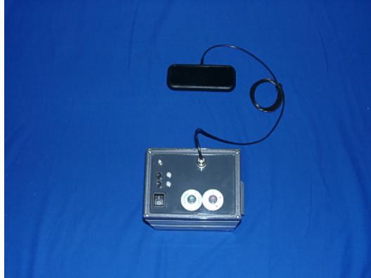
Figure 2: Connection of Sender Antenna
