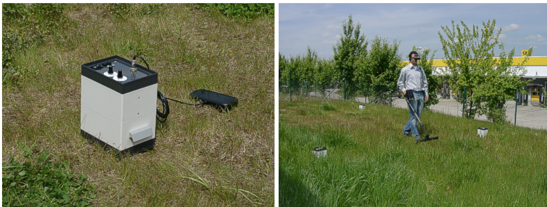
Figure 4: Placement of the VLF sender on a site
