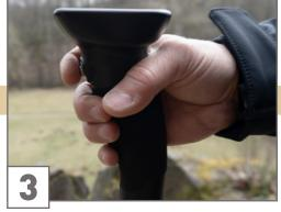
After finishing your 360° rotation, press the Trigger on the probe to finalize the calibration process.
