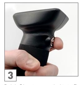
Push the Trigger to power on the detector. The Trigger LED turns **green** and the Minidisplay turns on.
