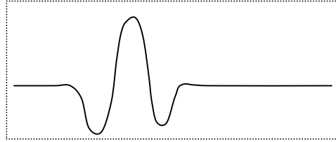
Fig. 2.2. Shape of an emitted electromagnetic wave
