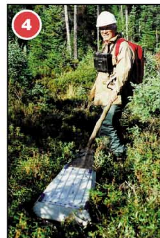
4. The Beep Antenna Beeps! A conductor has been localized.
