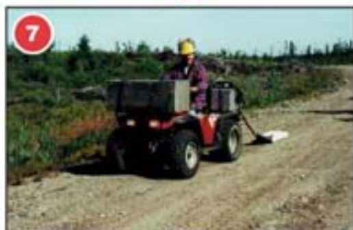
7. In the summer, an all-terrain vehicle carries the drill and the dynamite while the Beep Antenna surveys.
