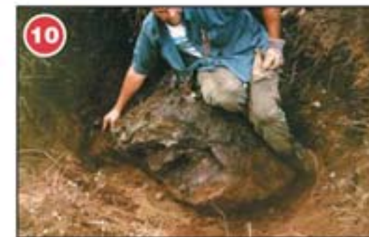
10. A worker sits on a float detected by the Beep Antenna and trenched. Four of the samples assayed averaged 2.97% Zn, 2.7% Cu, 30g/t Ag and 8g/t Au.
