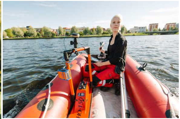
Cobra Plug-In GPR with the optional Smart Cart and operated from a Zodiac boat. (Using high accuracy GPS, SXBlue II GNSS, for positioning).
