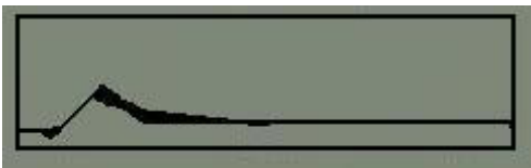
Small, shallow, low magnetic ferrous target
