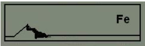
Small, shallow, strongly magnetized ferrous target
